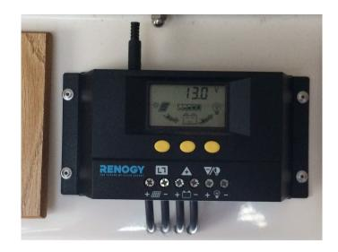
My research tells me that most charge controllers pulse the output at a high frequency when the battery approaches full charge. This produces audio noise and is a problem for ham operators. My solution is to temporarily reset the voltage above or below the noise threshold.
