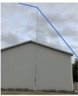
The balun, coax and wires were attached, the tubing extended and locked into place and the antenna hoisted into the air. I used a pine tree on each side of the pole to attach the wires in an inverted V. I also guyed the tubing in two locations to prevent it from swaying in the wind. In the photo I drew in the antenna wires since they do not show in the picture.
